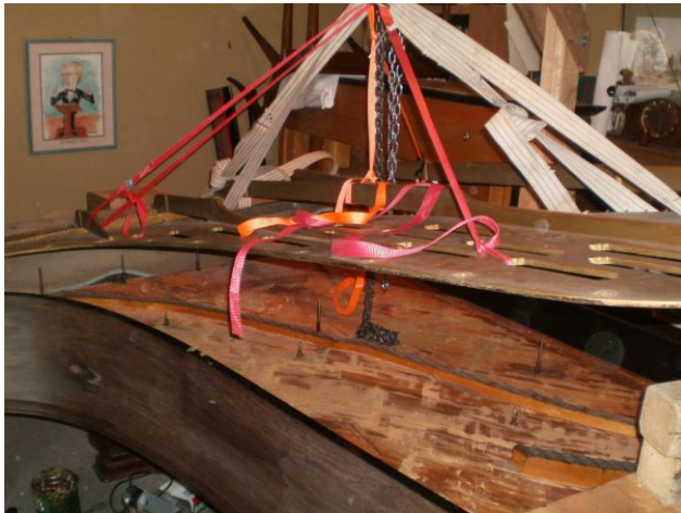
Two views of the 112-year old Burlock-Decker concert grand, first at an early stage of rebuilding, with the steel frame lifted to allow repair and refinishing of the soundboard, and then in St. George's Cathedral following its first public concert in a century, L to R, curator and restorer (and organist) John Hall, with past and present owners Irene Burlock of Virginia, and Warren Seale of Oakville, Ontario.
